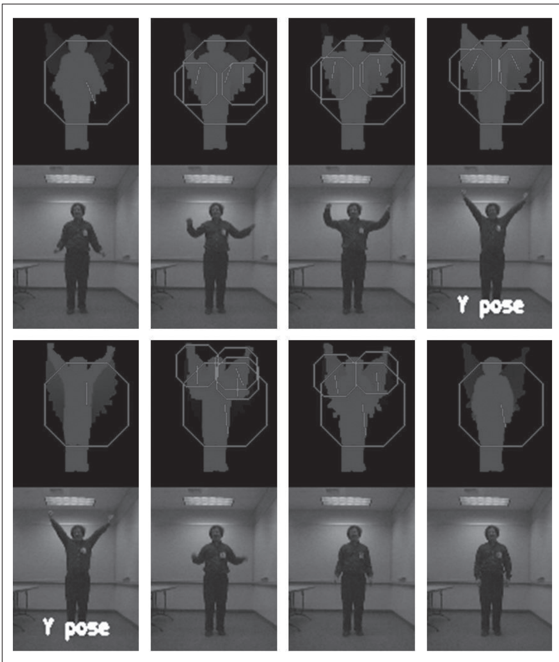
Figure 10-17. Results of motion template routine: going across and top to bottom, a person moving and the resulting global motions indicated in large octagons and local motions indicated in small octagons; also, the “Y” pose can be recognized via shape descriptors (Hu moments)
