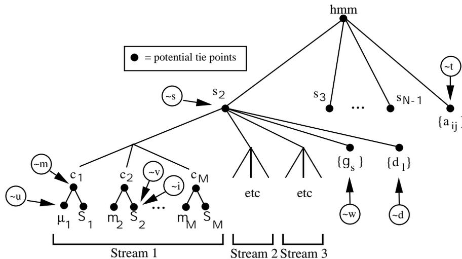
Fig. 7.8 HMM Hierarchy and Potential Tie Points
