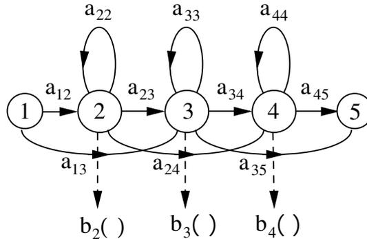
Fig. 7.1 Simple Left-Right HMM
