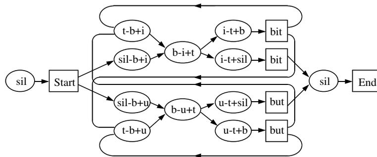
Fig. 12.10 Cross-Word Triphone Expansion of Bit-But Network
