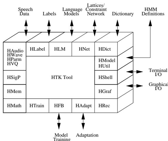
Fig. 2.1 Software Architecture
