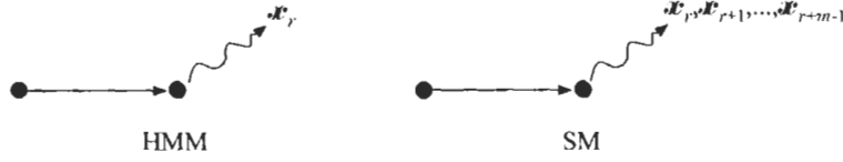
FIGURE 9.7: HMM and segment modeling (SM) for the emission of observations upon arrival of a transition at a state.
