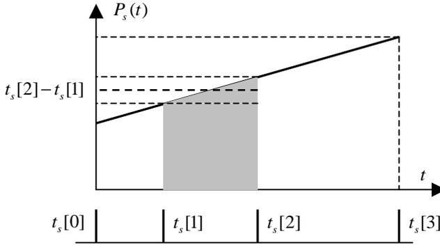
**Figure 16.11** The desired pitch period  $P_s(t)$  is a linearly increasing function of time such that the pitch period is doubled by the end of the segment. The four synthesis epochs  $t_s[j]$  are computed to satisfy Eq. (16.15). In particular,  $t_s[2]$  is computed such that  $t_s[2]-t_s[1]$  equals the average pitch period in that region. Note that the growing spacing between epochs indicates that pitch is growing over time.
