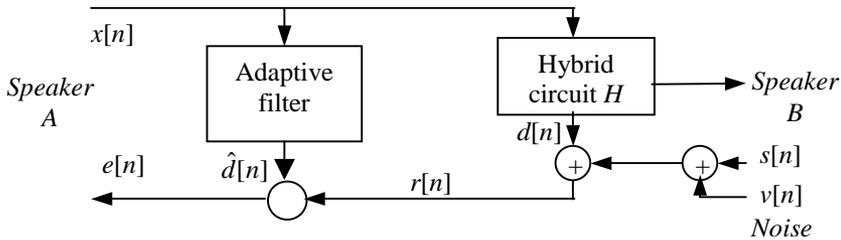
**Figure 10.18** Block diagram of echo canceling for a telephone communication.  $x[n]$  represents the remote call signal,  $s[n]$  the local outgoing signal. The hybrid circuit  $H$  does a 2-4 wire conversion and is nonideal because of impedance mismatches.
