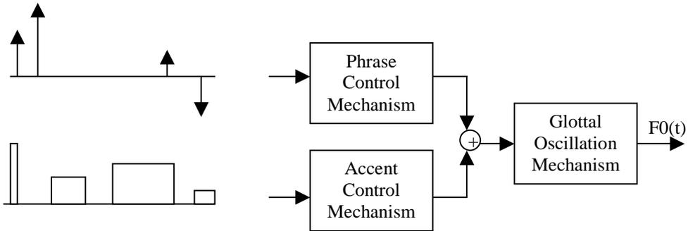
**Figure 15.10** Fujisaki pitch model [15].  $F_0$  is a superposition of phrase effects with accent effects. The phrase mechanism controls things like the declination of a declarative sentence or a question, whereas the accent mechanism accounts for accents in individual syllables.
