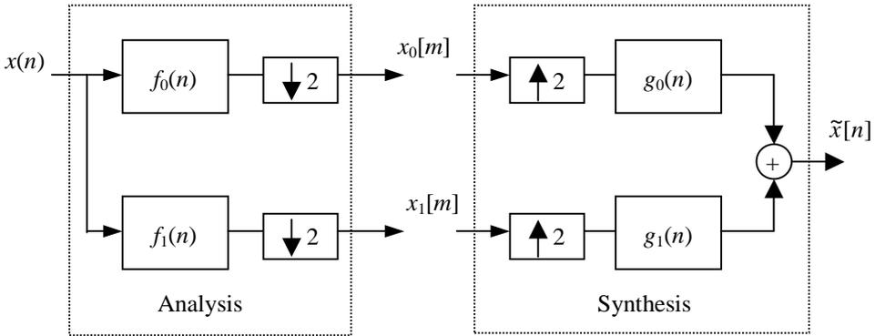
Figure 5.32 Two-band filterbank.
