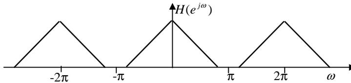
**Figure 5.8**  $H(e^{j\omega})$  is a periodic function of  $\omega$ .
