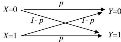
**Figure 3.18** A binary channel with two symbols.
