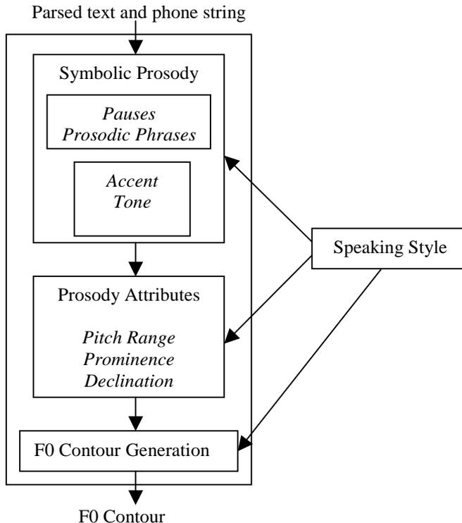
**Figure 15.3** Pitch generation decomposed in symbolic and phonetic prosody.
