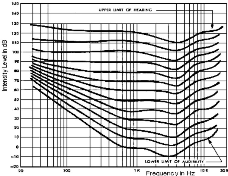
**Figure 2.11** Equal-loudness curves indicate that the response of the human hearing mechanism is a function of frequency and loudness levels. This relationship again illustrates the difference between physical dimensions and psychological experience (after ISO 226).
