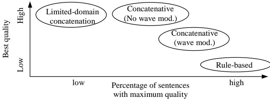
**Figure 16.1** Quality and task-independence in speech synthesis approaches.
