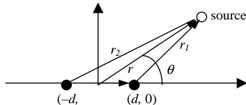
**Figure 10.10** Approximation to the noise-canceling microphone of Figure 10.9.
