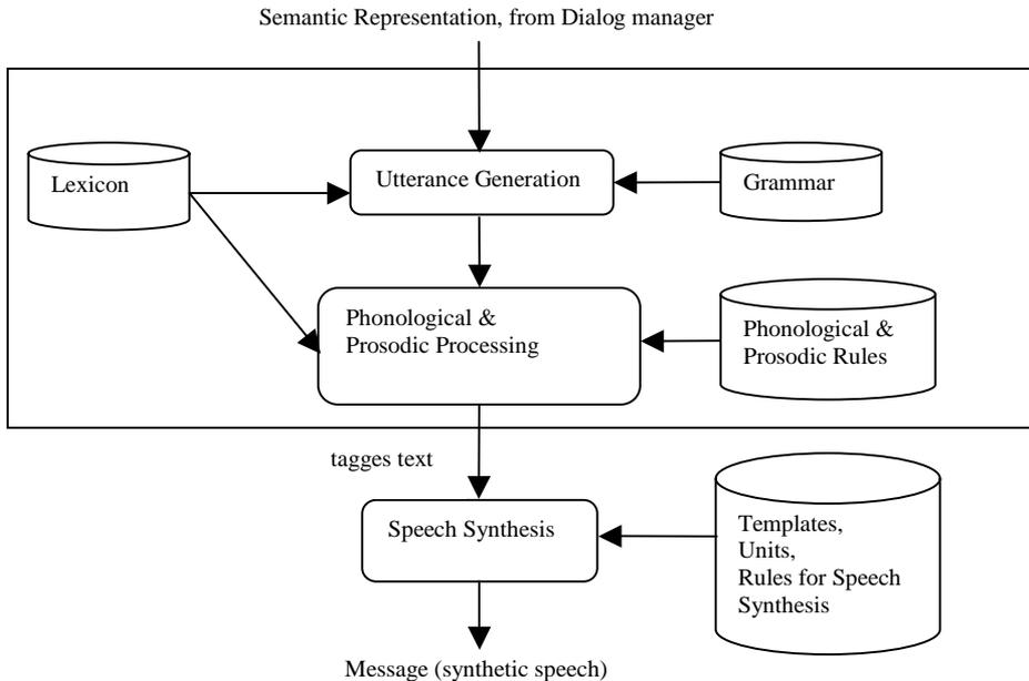
**Figure 17.26** Subsystems of message generation and rendition.
