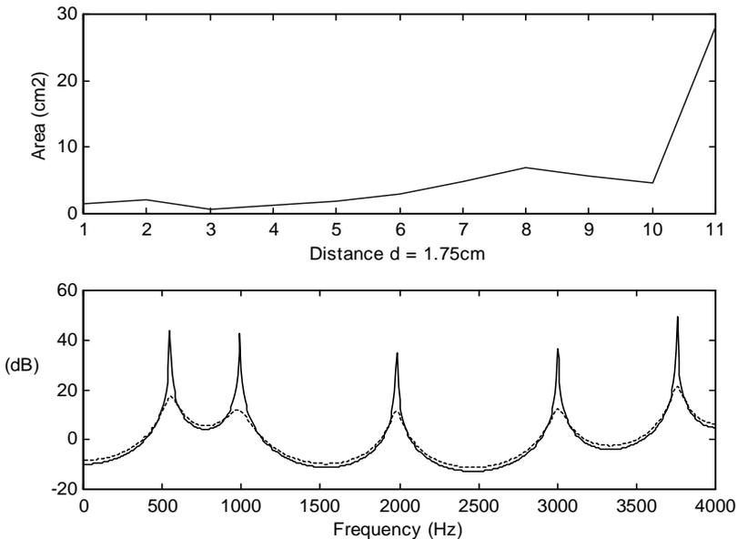
**Figure 6.11** Area function and frequency response for vowel /a/ and its approximation as a concatenation of 10 lossless tubes. A reflection coefficient at the load of  $k = 0.72$  (dotted line) is displayed. For comparison, the case of  $k = 1.0$  (solid line) is also shown.
