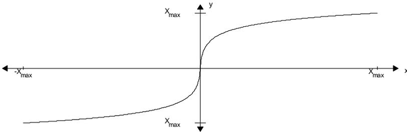
**Figure 7.2** Nonlinearity used in the  $\mu$ -law compression.
