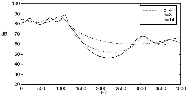
**Figure 6.21** LPC spectra of Figure 6.20 for various values of the predictor order  $p$ .
