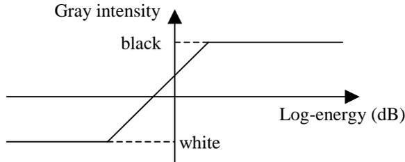
**Figure 6.6** Conversion between log-energy values (in the  $x$ -axis) and gray scale (in the  $y$ -axis). Larger log-energies correspond to a darker gray color. There is a linear region for which more log-energy corresponds to darker gray, but there is saturation at both ends. Typically there is 40 to 60 dB between the pure white and the pure black.
