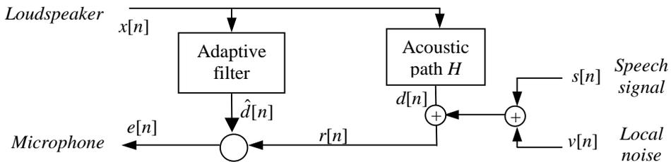
**Figure 10.17** Block diagram of an echo-canceling application.  $x[n]$  represents the signal from the loudspeaker,  $s[n]$  the speech signal,  $v[n]$  the local background noise, and  $e[n]$  the signal that goes to the microphone.
