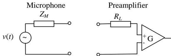
**Figure 10.6** Electrical equivalent of a microphone.
