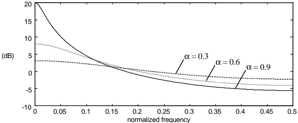
**Figure 5.25** Magnitude frequency response of the first-order IIR filter.
