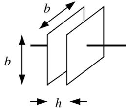
**Figure 10.5** A diagram of a condenser microphone.
