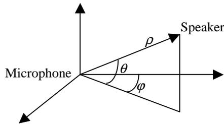
**Figure 10.21** Spherical coordinates  $(\varphi, \theta, \rho)$  with  $\varphi$  being the direction of arrival,  $\theta$  the elevation angle, and  $\rho$  the distance to the reference microphone.
