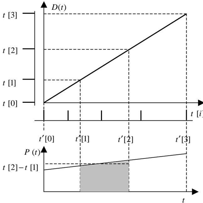
**Figure 16.13** Time-scale modification of speech. The five analysis epochs  $t_a[i]$  are shown in the  $x$ -axis and the four synthesis epochs  $t_s[i]$  in the ordinate. Duration is shortened by 25% while maintaining the same pitch period. The corresponding virtual analysis epochs  $t'_a[i]$  are obtained through the mapping  $D(t)$ , a linear transformation with  $\alpha = 0.75$ .
