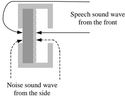
**Figure 10.13** Cross section of a unidirectional microphone.
