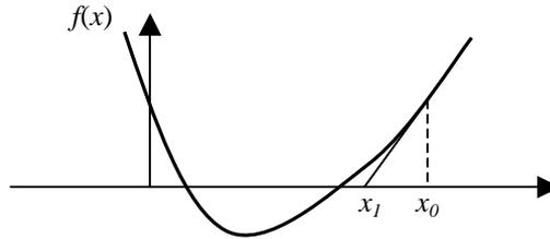
**Figure 10.20** Newton-Raphson method to compute the roots of a function.
