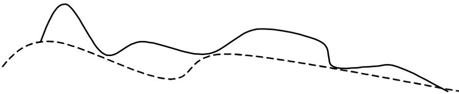
**Figure 15.11** Composite contour obtained by low-pass filtering the impulses and boxes in the Fujisaki model of Figure 15.10.
