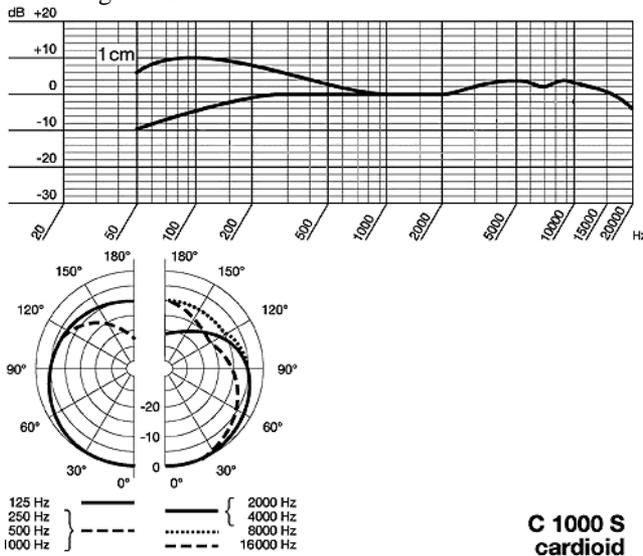
**Figure 10.15** Characteristics of an AKG C1000S cardioid microphone: (a) frequency response for near and far field conditions (note the proximity effect) and (b) polar pattern for different frequencies.
