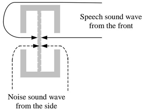
**Figure 10.9** Cross section of an ideal bidirectional microphone.
