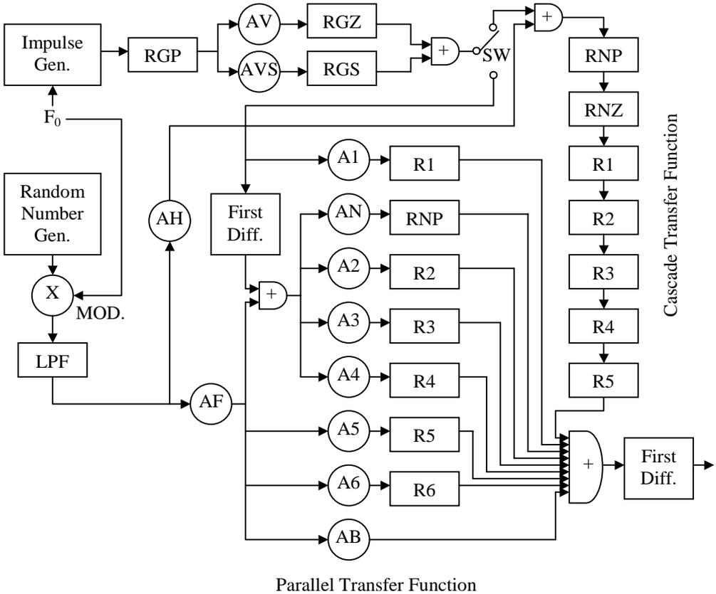
Figure 16.3 Block diagram of the Klatt formant synthesizer (after Klatt [4]).
