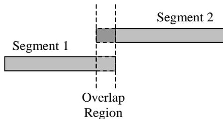
**Figure 16.7** Measurement of the spectral discontinuity in the overlap region. The dark gray area is the speech region that precedes segment 2 and does not form part of segment 2. This area should match the last part of the segment 1.
