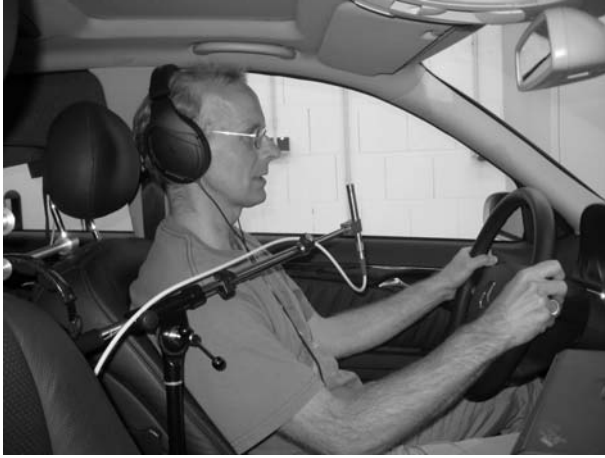
Fig. 10.19. Setup for Lombard speech recordings.
