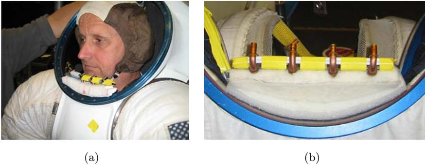
**Fig. 12.13.** Illustration of two equispaced, linear microphone arrays and their mounting apparatuses developed in the multichannel acoustic data collection experiments. (a) The SMS array mounted in a Mark III suit and (b) the Pro-Audio microphone array mounted in a REI suit.
