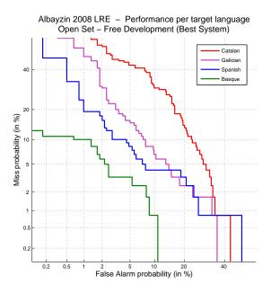
Figure 5: DET curves for target languages, using the best system in the OF test condition.
