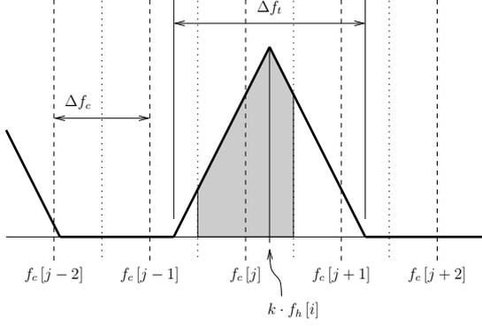
Figure 1: Riemann sampling of the  $k$ th idealized harmonic of the continuous-frequency comb for fundamental frequency  $f_h [i]$ . Shown in gray is the area assigned, during filter construction, to the  $j$ th element of the corresponding discrete-frequency comb filter  $\mathbf{h}_i$ . Frequency shown along the  $x$ -axis; symbols as in the text.
