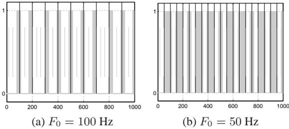
Figure 2: Discrete-frequency comb filters  $\mathbf{h}_i$ , in gray, produced by Riemann sampling of continuous-frequency filters  $h_i(f)$ , in black, with triangular harmonics of base width  $\Delta f_t \rightarrow 0$ . The example in (b) violates the Nyquist quefrequency criterion; that in (a) does not.
