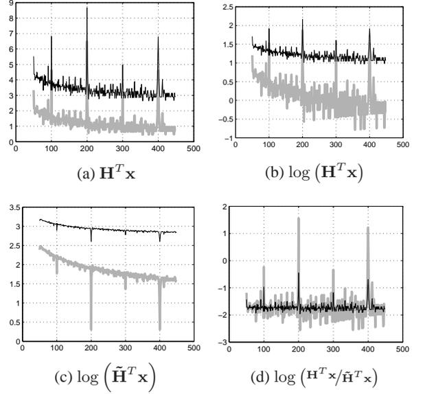
Figure 3: Various intermediate representations leading to Equation 3. The idealized spectrum  $\mathbf{x}$  was formed by adding a column of  $\mathbf{H}$ , that corresponding to  $F_0 = 200$  Hz, to white noise. Gray denotes a SNR of 10, black that of 1.
