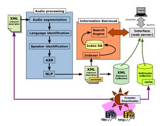
Figura 1. The architecture of the SDR system.
