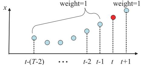
Fig. 3. Calculation of dynamic features for pedal operation signals using Eq.(3).
