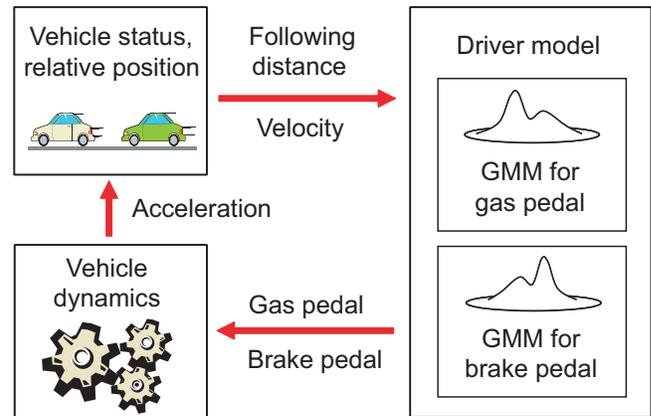
Fig. 1. Cyclic process of driving signal generator.
