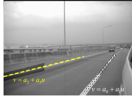
Fig. 13. Adaptive ROI of far lane marking.
