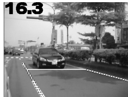
Fig. 20. The detection results for road.
