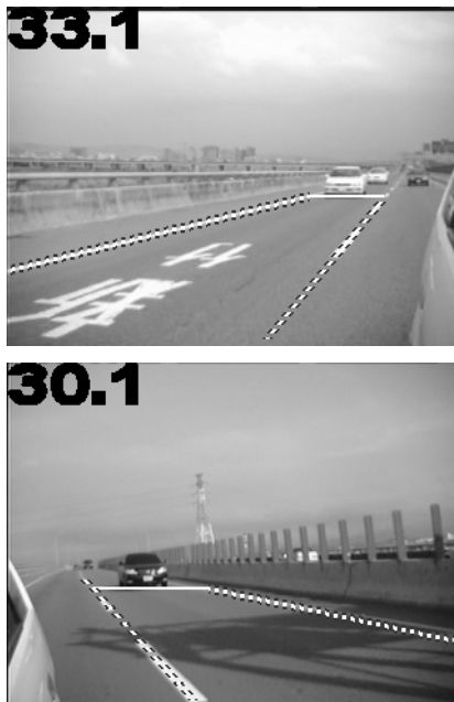
Fig. 21. The detection results for highway.
