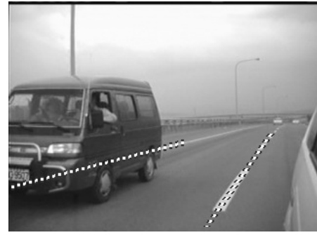
Fig. 19. The estimated far lane marking.
