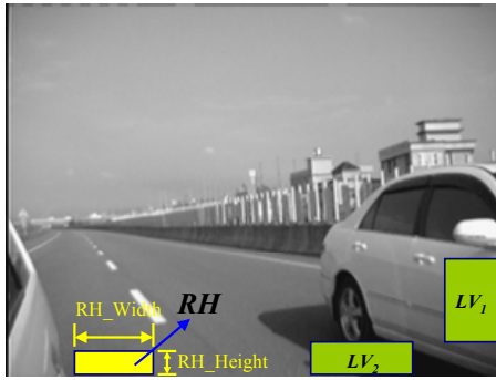
Fig. 11. The check region of vehicle detection in the neighboring lane.
