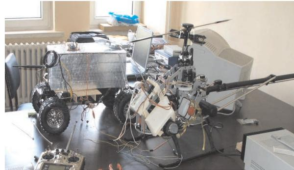
Fig. 1. The hardware-in-the-loop tests[7] of the micro-avionics core design. The avionics pod is placed on the 1/6 RC Humvee, which is used at the field tests. The servo lines are connected to the Vario Microhelicopter with the helicopter mathematical model running on a xPC target.
