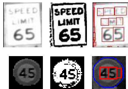
Fig. 6. Illustration of the character segmentation procedure in a rectangle (U.S. case, top line), and in a circle (E.U. case, bottom line): the searched area (left) is first binarized by adaptive thresholding (middle), the connected-component labeling is applied for finding potential digits (right)
