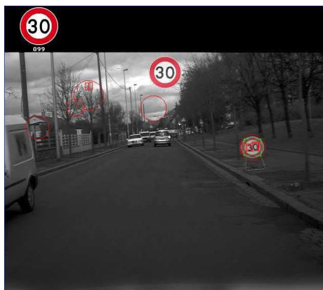
Fig. 9. Example of speed-limit sign detection on a E.U. street. All detected circles are shown (in red), and the candidate digits segmented inside them are outlined in red. The speed signs recognized on the current image are shown on the top black zone, with their associated confidence, and the currently validated speed limit is superimposed on top-center of image.
