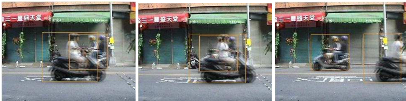
Fig. 4. Multiple object tracking with occlusion (two motorcycles).
