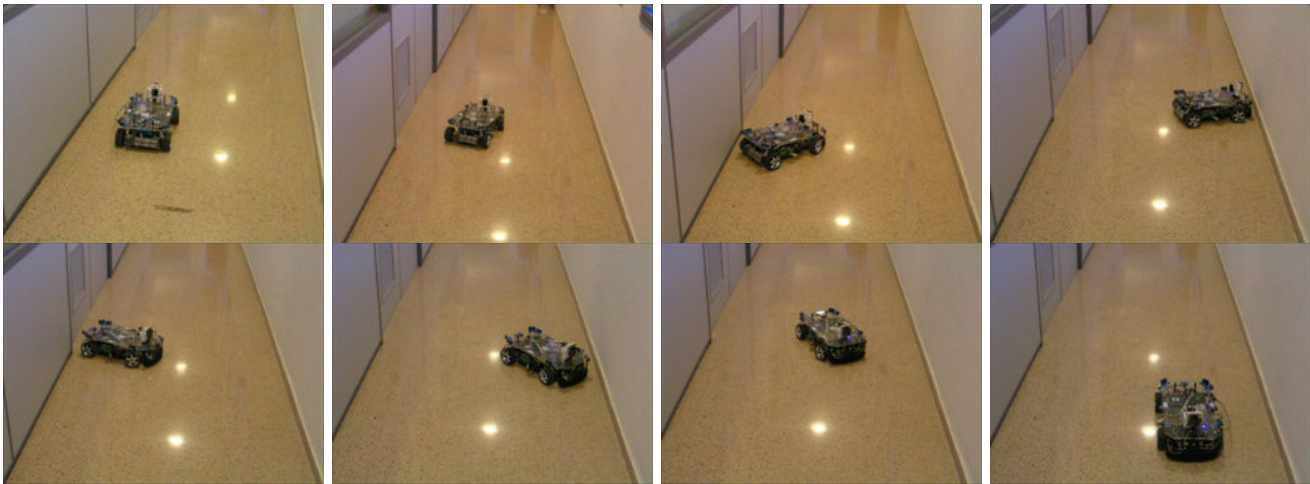
Fig. 6. Sequence of images showing the wall following behaviour with a virtual wall closing the corridor.
