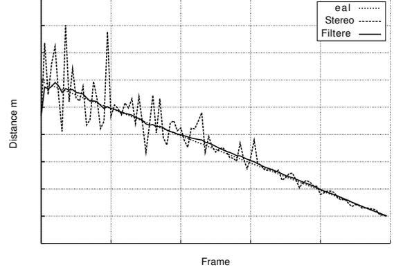
Fig. 3. Estimation results of the presented Kalman filter. The considered world point is at the initial position  $(10.0 \text{ m}, 1.0 \text{ m}, 60.0 \text{ m})^T$ . The observer moves at a constant speed of  $v_z = 10 \frac{\text{m}}{\text{s}}$  in positive  $z$ -direction (20 fps).
