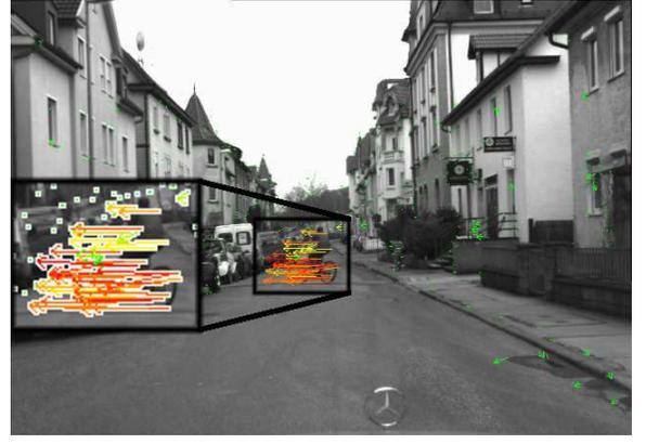
Fig. 7. Velocity estimation results with image based ego-motion compensation.
