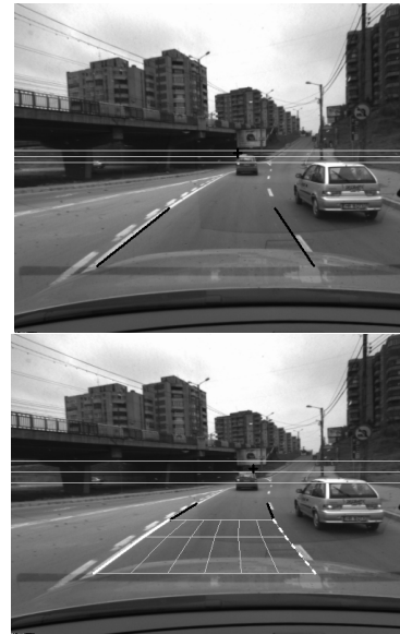
Fig. 4. Updating the clothoidal lane profile from linear segments using the Extended Kalman Filter
