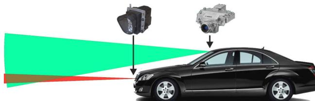
Fig. 1. Sensor mounting points and fields of view for the sensorfusion setup combining multibeam lidar and monocular vision.
