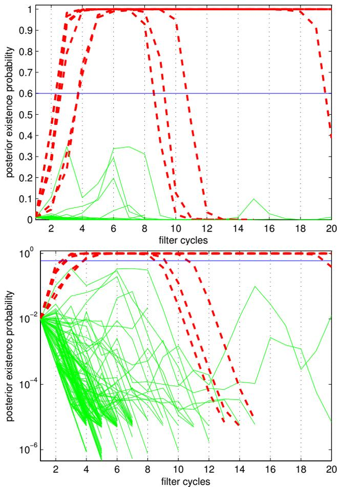
Fig. 11. Temporal evolution of the IPDA estimated posterior probabilities of existence for several true positive (red) and false positive (green) tracks in linear (top) and logarithmic scale (bottom). Tracks are confirmed and pruned by thresholding the existence probability. A possible track confirmation threshold is represented by the blue line.
