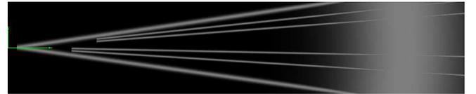
Fig. 8. Objects can only appear and vanish near the borders of the FOV and occlusion areas. The resulting probability interval  $[0..1]$  is color mapped from black to white.
