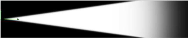
Fig. 4. Object persistence probability related to the sensor field of view of  $16^\circ$ , given the position in vehicle coordinates (green). The probability interval  $[0..1]$  is color mapped from black to white.
