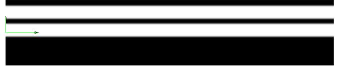
Fig. 6. Persistence probabilities from digital map of a two lane highway. As objects can only be on the road, all other areas have probability zero. The probability interval  $[0..1]$  is color mapped from black to white.
