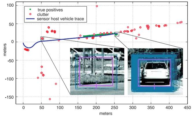
Fig. 3. Time accumulated birdview of a drive through a complex urban scene. The blue line is the trace of the sensor host vehicle, with sensed true positive measurements from three other cars (green boxes) and false positive readings in the background (red dots).
