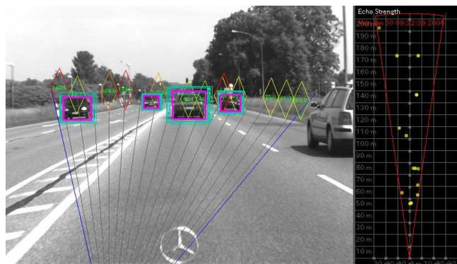
Fig. 2. Vehicle detection scheme. The lidar echoes (yellow dots in right birdview) are projected into the image domain (diamonds on gray rays in left video image). An image classifier is applied on lidar projections (cyan boxes). A detection box cluster algorithm outputs the final detections (magenta boxes).
