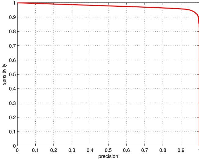
Fig. 9. Vehicle detection receiver operating characteristics (ROC) resulting from the variation of the detection decision threshold.
