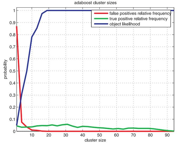
Fig. 10. Relative frequency of detection cluster sizes given the target exists (green) and given the target does not exist (red) and resulting cardinal existence probability  $p_c^{TP}(z_i)$  (blue).
