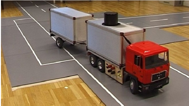
Fig. 11. Truck with one-axle trailer model (t2) executing a parallel parking maneuver.
