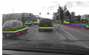
Fig. 5. Coordinate transformation: The measurements of the laser scanner as well as corresponding object features can be transformed to the video coordinate system due to calibrated and synchronous sensors. The example shows the transformed laser scanner measurements in the image.
