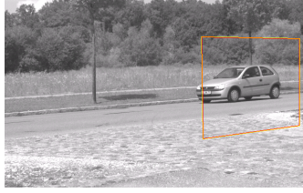
Fig. 7. Video ROI: An appropriate side of the object cuboid, which is estimated by the laser scanner, is transformed to the video image. The side is increased to contain some amount of background pixels around the object.
