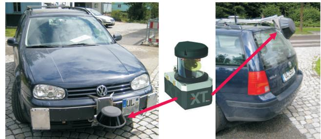
Fig. 1. *Left:* Horizontally mounted ALASCA XT laser scanner. *Right:* Vertically mounted ALASCA XT laser scanner.
