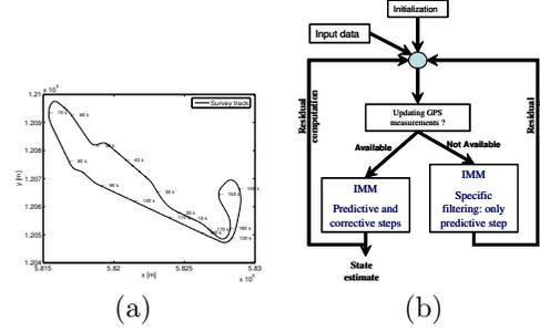
Fig. 2. (a): Survey track, (b): Localization system based on IMM
