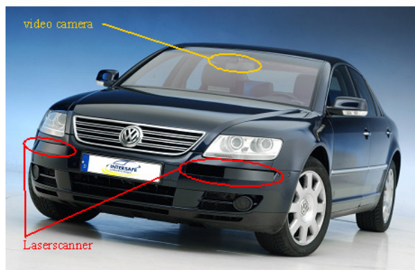
Figure 1: Sensor integration in the Phaeton demonstrator.
