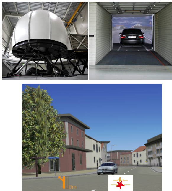
Figure 3: BMW dynamic driving simulator.
