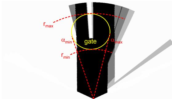
Fig. 6. Occlusion probability: The occlusion detection calculates occlusion probabilities of discrete areas. These probabilities are displayed as in Figure 4 (white: certainly occluded, black certainly not occluded). The occlusion probability of a received object is calculated by integration of the occlusion probabilities under the assumed Gaussian pdf in the elliptical gate.
