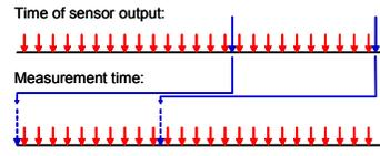
Fig. 4. GPS latency: The output of the GPS receiver (blue arrows) corresponds with a measurement time several hundred milliseconds ago. Therefore, the GPS measurements are older than the last velocity and yaw rate measurements (red arrows).
