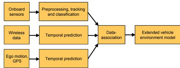
Fig. 2. System overview: The system performs tracking and classification of objects, which are observed by onboard sensors. Object information obtained from wireless communication is filtered to predict the object state to the time of the current sensor measurements. In addition, the host vehicle's position has to be predicted. The data association algorithms fuse information of all sources and provide the extended vehicle environment model.
