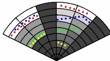
Fig. 5. Occlusion detection: The algorithm estimates occlusion probabilities of discrete areas in polar coordinates based on the four horizontal layers of the laser scanner. The probabilities are indicated by gray values between black (not occluded) and white (occluded). The circles are sensor measurements. The corresponding layer is indicated by color. The occlusion probability of an area rises with the number of layers with corresponding measurements between the area and the sensor (center).
