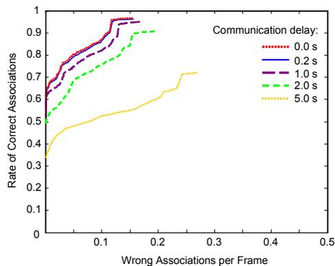
Fig. 8. Results: Several simulated communication delays were compared. The plots show the rate of correct associations over the mean number of wrong associations per frame. Different combinations of the measures are obtained by changes of the threshold for the minimum accepted association probability.
