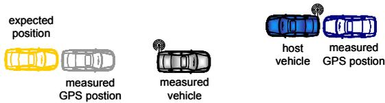
Fig. 3. Position error, caused by measurement and transmission delay: Usually the received positions and the last GPS position of the host vehicle correspond to past sensor measurements. If the received position is used directly, the object will be expected very far away from its correct position. Therefore, the received information and the host vehicles position have to be predicted to the current time.
