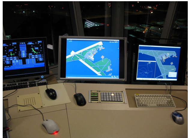
Fig. 3. Dispatchers CaMNA display unit (central) installed within active displays of airport management center - for pilot tests, only.
