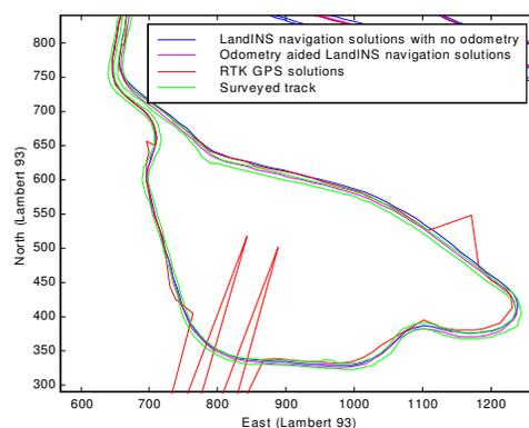
Fig. 5. GPS real-time rejection filter in the forest
