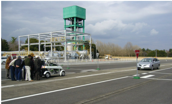
Fig. 8: A scene of the experiments: the single seat vehicle is making right turning and the oncoming passenger car is going straight.
