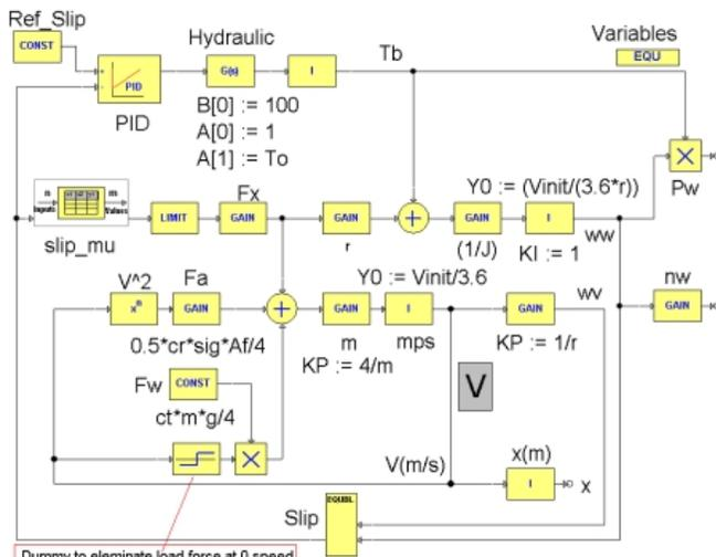
Fig. 6. Integration of hydraulic ABS to QCM
