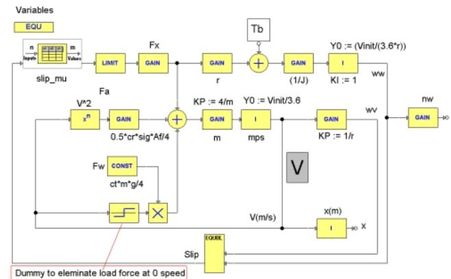
Fig. 4. Quarter car model during braking
