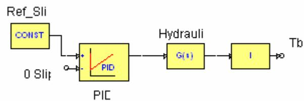
Fig. 5. Hydraulic ABS model
