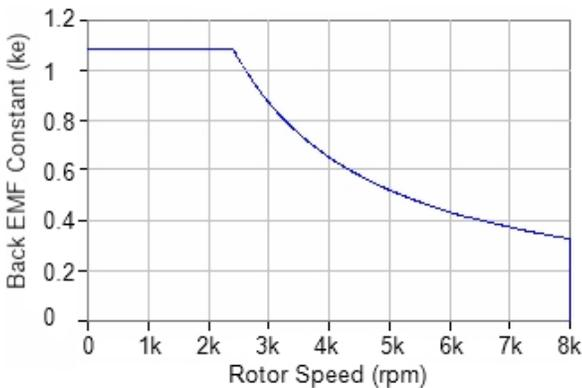
Fig. 11. Rotor Back EMF constant calculated in Flux\_Calc Block shown in Fig. 9
