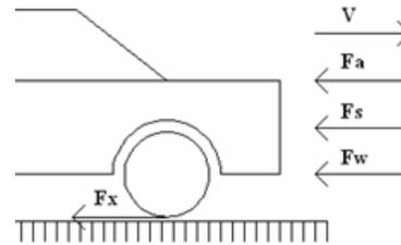
Fig. 1. Forces acting on the vehicle.
