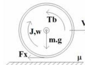
Fig. 2. Wheel longitudinal dynamics
