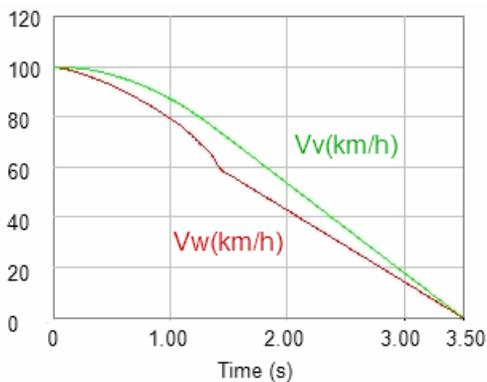
Fig. 7. Vehicle (Vv) and wheel (Vw) speeds vs. time simulation result for hydraulic braking.
