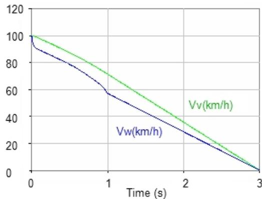
Fig. 13. Vehicle (Vv) and wheel (Vw) speeds vs. time simulation result for regenerative braking.
