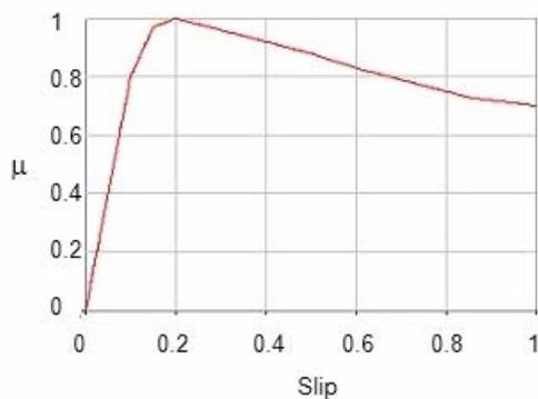
Fig. 1.  $\mu$  - slip curve used for tire modeling
