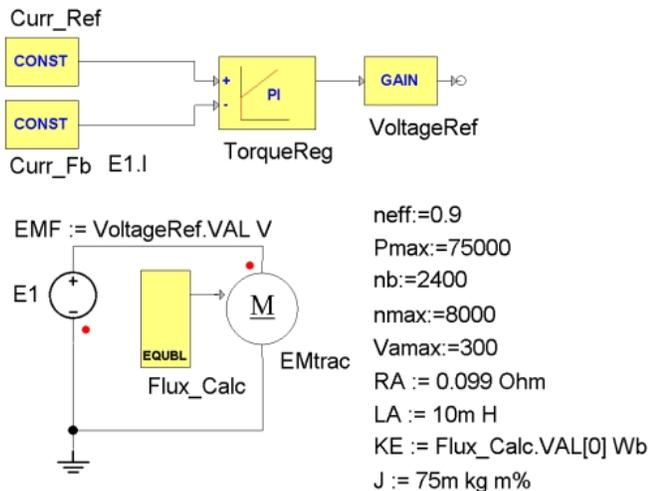
Fig. 9. Modified dc motor and torque loop model
