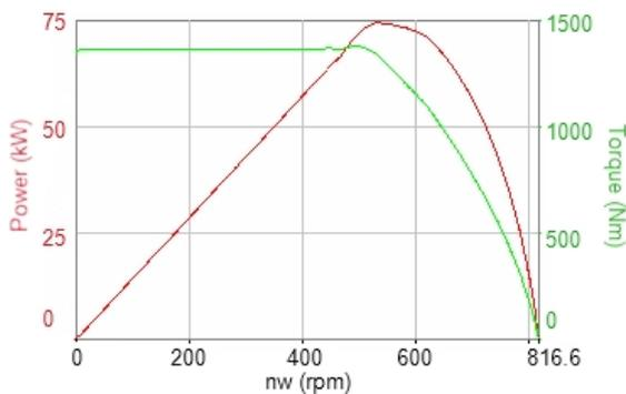
Fig. 8. Braking power and torque vs. wheel rotational speed (nw)
