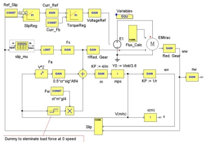
Fig. 12. QCM modified for regenerative ABS braking
