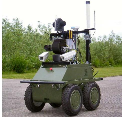
Fig. 1. An image of the EyeRobot robot vehicle demonstrator. The two white cameras are a stereo pair that can be used for obstacle detection. Between these cameras is a pan-and-tilt unit which carries several cameras, microphones and a range finder for remote surveillance tasks.
