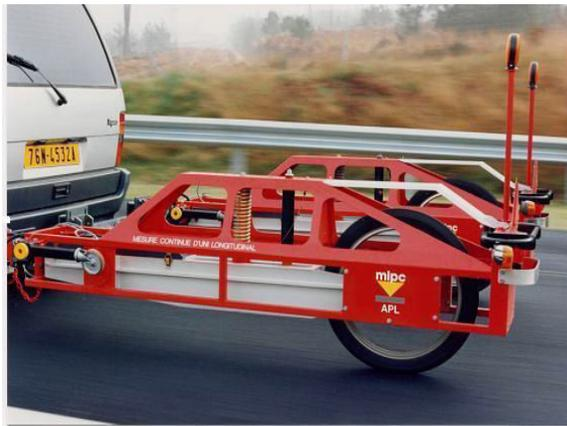
Fig. 3. Longitudinal Profile Analyser (APL in french)
