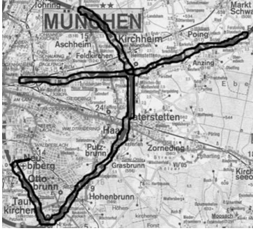
Fig. 1. Test track: Highway intersection in the South-West of Munich (Germany) with two and three lanes, respectively. The distance was covered twice by every participant, first without ACC ( \bar{X} 59 \pm 5 min) and afterwards with ACC ( \bar{X} 58 \pm 3 min).
