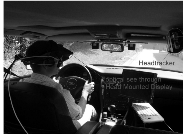
Fig. 5: HMD and headtracker integrated at the Vehicle in the Loop
