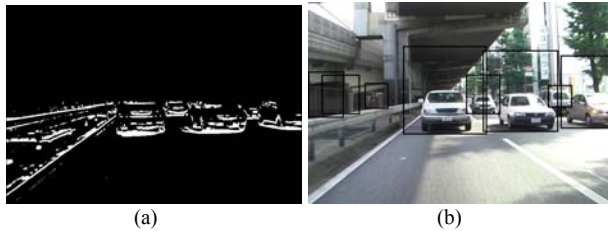
Fig. 1. (a) Gradient image of shadow underneath vehicles (b) ROI
