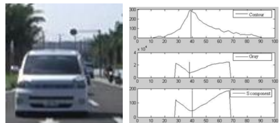
Fig. 2. Computing the three kinds of symmetry axes
