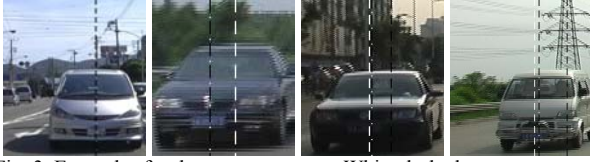
Fig. 3. Examples for the symmetry axes. White dashed represents gray symmetry axis; Black dashed represents binary value symmetry axis; Dash-dot represents S component symmetry axis
