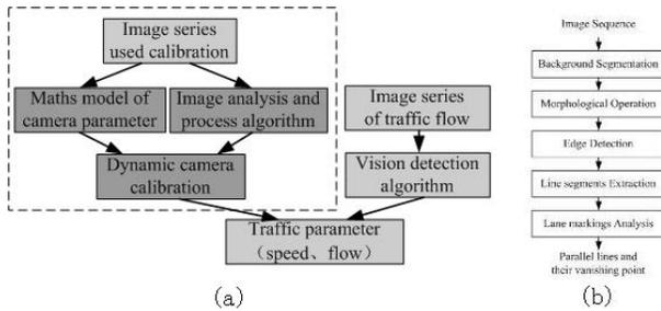
Fig. 5. (a) The process chart of this dynamic algorithm; (b) The process chart of the lane markings detection algorithm
