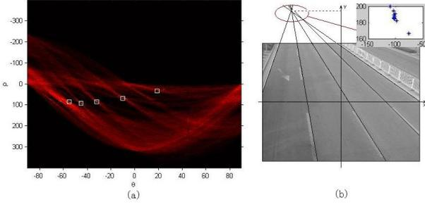
Fig. 8. (a)Hough transform for the Fig.7(b); (b) result of lane detection in traffic image through some image processing algorithms
