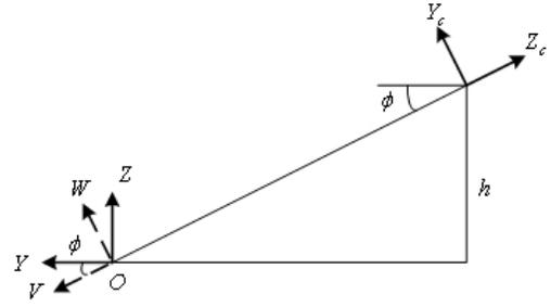
Fig. 2. The plane figure constituted by the lens's main axis and the perpendicular line from camera to ground plane
