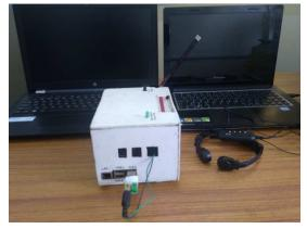
Figure 1: Set-up for Praat-based voice analysis using acoustic and throat microphones
