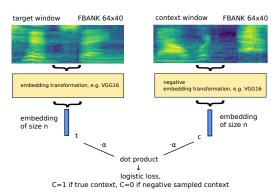
Figure 3: Unspeech embeddings are trained using a Siamese neural network architecture combined with a dot product. We use the VGG16A network as embedding transformation in the yellow boxes (a convolutional neural network with 16 layers).
