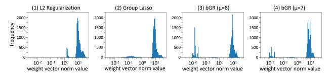
Figure 2: Histogram of each column vector norm value in all weight matrices as the model parameters. The distributions towards the left side are unneeded so the corresponding nodes can be pruned. The proposed bGRs method can safely prune DNN nodes than the other approaches.
