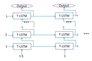
Figure 1: Flowchart of multi-layer time-LSTM (T-LSTM). The output of a T-LSTM is used as the input of the T-LSTM at the same time step in the next layer and the recurrent input of the T-LSTM at the next time step in the same layer.
