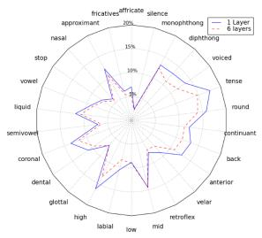
Figure 2: *The error rate of the speech attribute detectors when using 1 layer and 6 layers*
