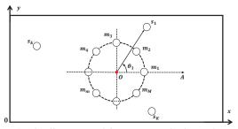
Figure 1: The illustration of the geometrical relationship. Here, an equispaced circular sensor array consists of M microphones and K sources move around the array.
