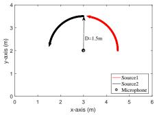
Figure 4: The trajectories of two sources in the simulated environment. The two sources move around the array with a fixed velocity. Here the angular separation of two sources is  $90^{\circ}$ .
