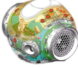
Figure 1: Head of the NAO robot with visible microphones highlighted in red (©Aldebaran Robotics).
