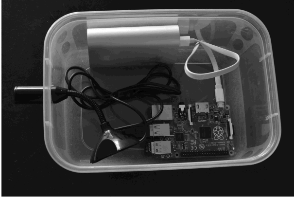
Figure 1: The Raspberry Pi based acoustic sensor system.
