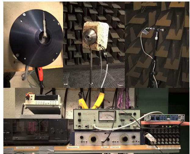
Figure 2: A snapshot of the recording devices. The top row shows B&K Type 4219 artificial voice along with G.R.A.S. Type 46AF free-field microphone. In the bottom row the amplifiers, A/D and D/A signal converters and filters are shown.
