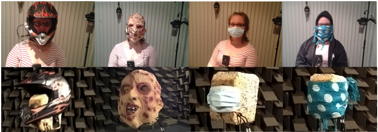
Figure 1: In the top row, a volunteer wears 4 different face masks: motorcycle helmet, rubber mask, surgical mask and scarf. The speech material under face mask is collected with support from Finnish National Bureau of Investigation and University of Helsinki. In the bottom row, we simulate the recordings with face mask inside anechoic chamber by using an artificial voice generator devised in a pretend dummy head.
