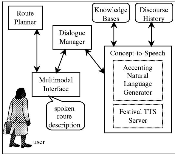
Figure 2: System Architecture.
