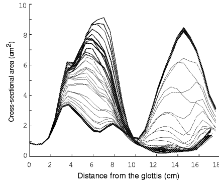
Fig. 6 Vocal tract area functions calculated from the physiological model for vowel sequence /iai/. Thin lines show the area functions during the transition between /i/ and /a/.
