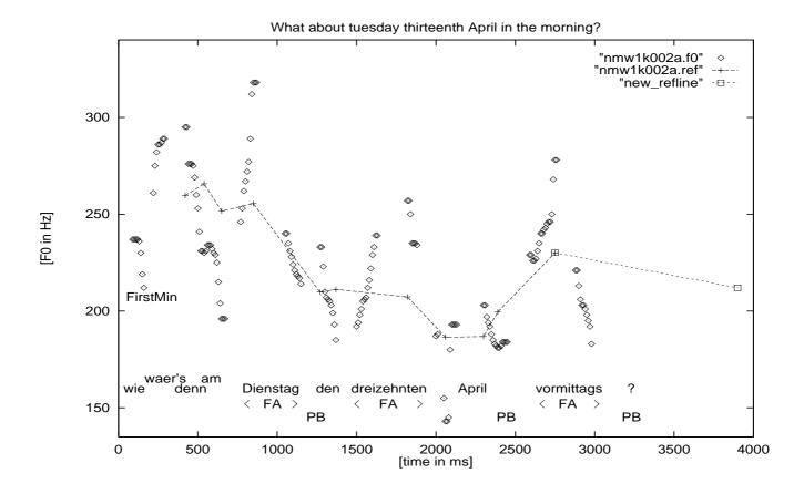
**Figure 1:**  $F_0$  contour extracted from a dialogue utterance (nmw1k002a.f0) with reference line (nmw1k002a.ref) and labelled focus accents (FA) and phrase boundaries (PB). For better recognition of focus accents in sentences with rising  $F_0$  contour the reference line was artificially extended (marked as 'new-refline').
