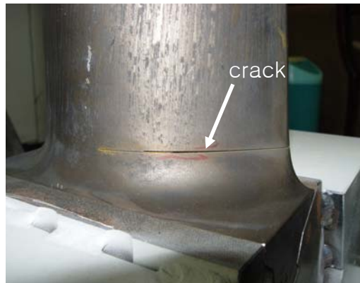
Figure 4 – Crack in the blade
