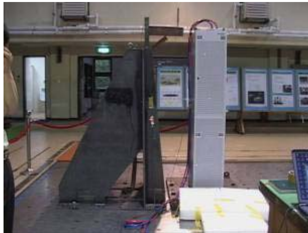
Photo 3 –Test setup of the Slim BTS in side-to-side direction
