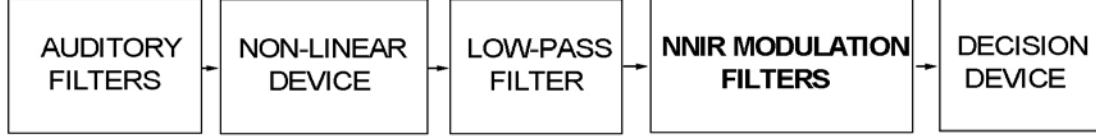
Fig. 3. Auditory pathway model of modulation perception and analysis used in the simulations (see the text for details).
