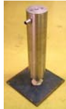
Figure 3 - Giant-Magnetostriction vibrator for Primary wave
